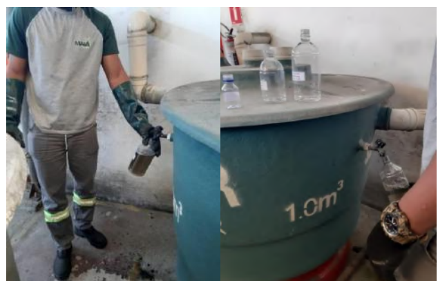
Fig. 3: (a) shows the time of collection of the raw influent; (b) the treated effluent. Source: Company's technical department of FIBROMAR.
