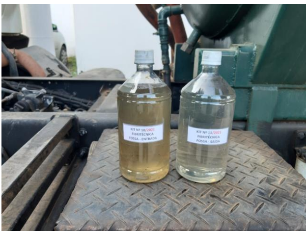
Fig. 4: Comparison of samples – On the left side the raw effluent and on the right side the treated effluent. Source: Prepared by the author (2021).
